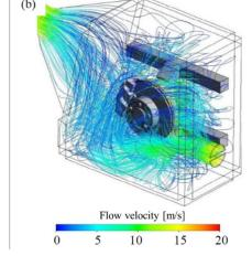
Investigation of particle **transport** efficiency  $\eta_m$  and particle uniformity  $U_n$ across the measurement tunnel diameter, where the particles sample is abstracted by the probe. (particle size range 0,1-4μm)
