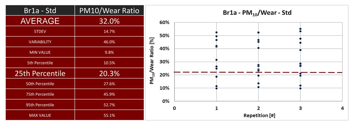
Labs with  $PM_{10}$ /Wear ratio lower than 20.3% might have underestimated the  $PM_{10}$  fraction
