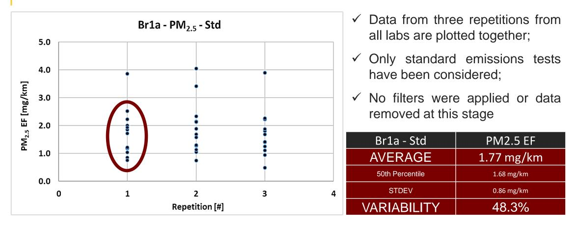
Unfiltered data show a variance of  $PM_{2.5}$  EFs between 0.5-4.1 mg/km at a brake level. This results in a high measurement variability of approximately 48% - Most data points are found between 1.0-2.0 mg/km
