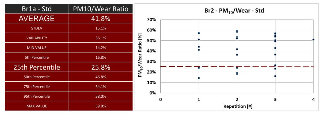
Labs with PM<sub>10</sub>/Wear ratio lower than 20.3% might have underestimated the PM<sub>10</sub> fraction
