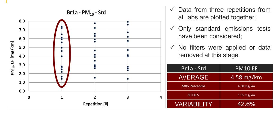
Unfiltered data show a variance of  $PM_{10}$  EFs between 1.4-7.9 mg/km at a brake level. This results in a high measurement variability of approximately 43%.
