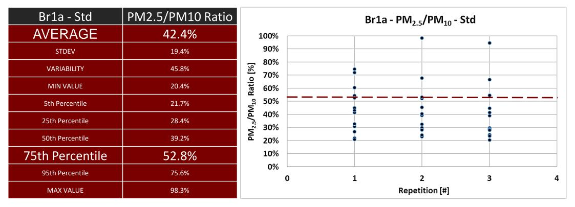
Labs with PM<sub>2.5</sub>/PM<sub>10</sub> ratio higher than 52.8% might have underestimated the PM<sub>10</sub> fraction
