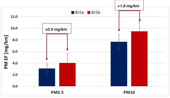
Error bars correspond to the SD of 12 measurements (4 Labs) – Variability of 1SD=17%
