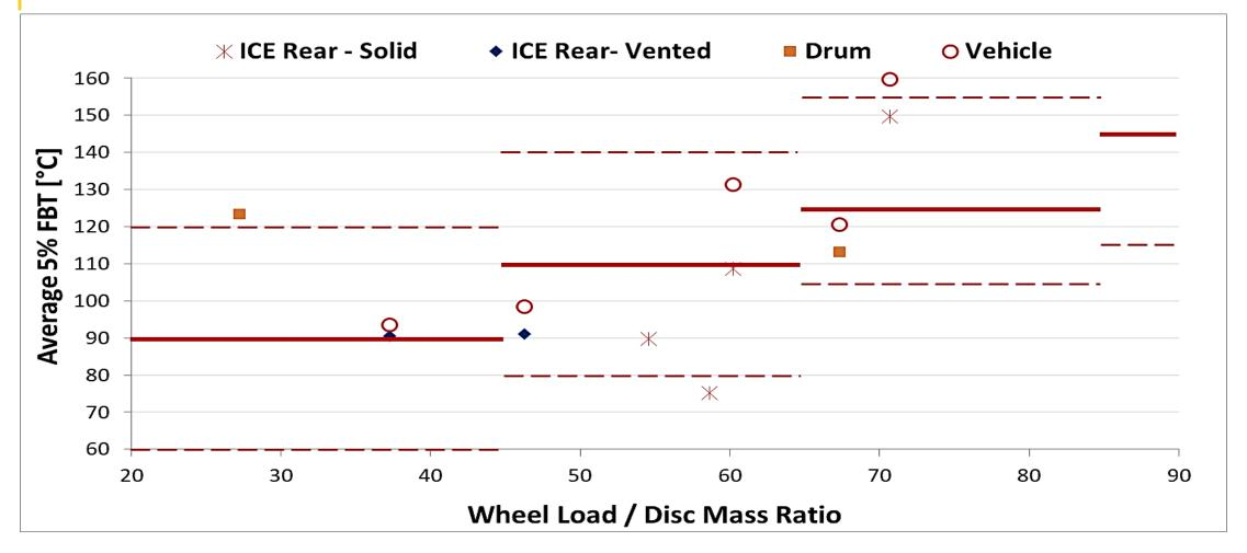
Similar observations as for average temperature – One vehicle data-point is outside the spec – More refined values are impossible to be derived
