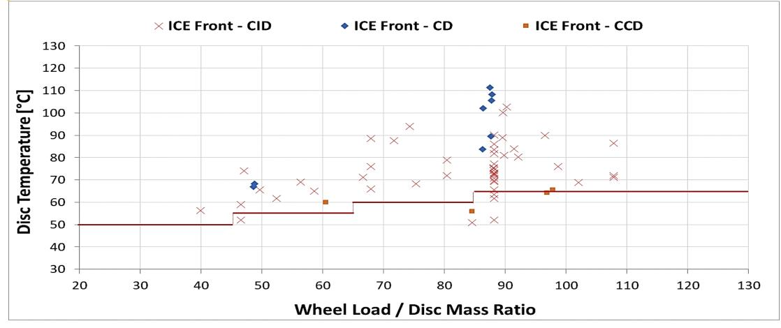
Average Trip #10 temperature has been succesfully applied during the ILS. it ensures that Labs are not running the test much cooler than they should – *No changes have been applied to the TF2 proposal regarding this criterion*
