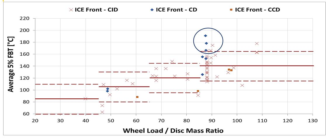
Average FBT has been generally succesfully applied during the ILS. it ensures that Labs are not running the test neither much cooler nor much hotter than they should – *There are non-compliances for the maximum threshold FBT for the 4th Group (WL/MD > 85)* – *This shall be corrected*
