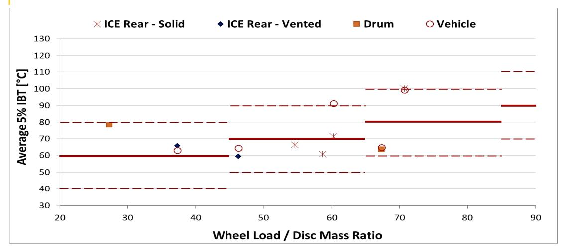
Similar observations as for average temperature – One vehicle data-point is borderline – Available dyno data all within the spec – More refined values are impossible to be derived
