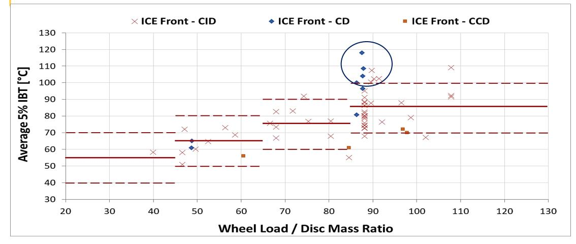
Average IBT has been generally succesfully applied during the ILS. it ensures that Labs are not running the test neither much cooler nor much hotter than they should – *There are non-compliances for the maximum threshold IBT for the 4th Group (WL/MD > 85) – This shall be corrected*
