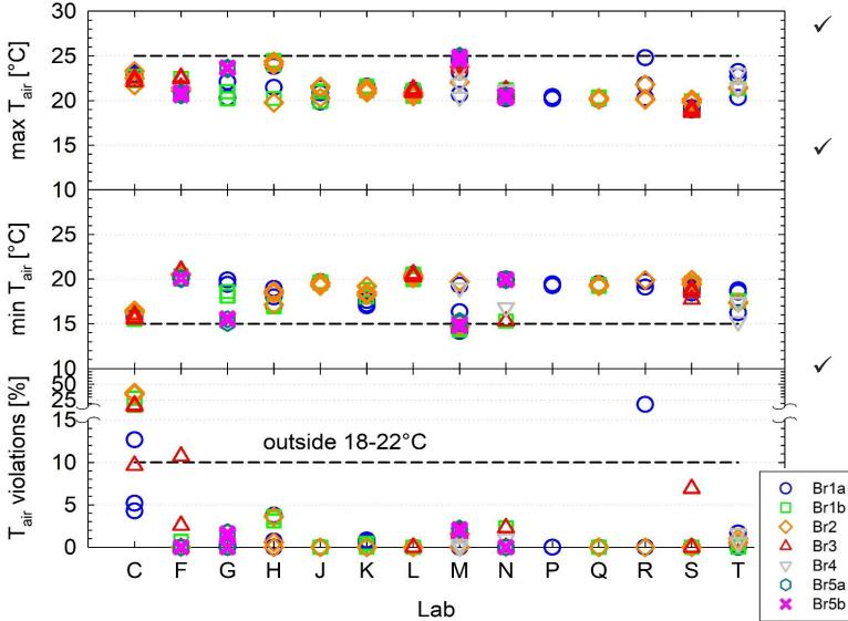
The TF2 protocol foresees that Labs shall run the tests with the cooling air conditioned at 20±2°C;
