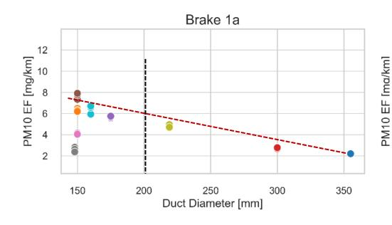
The ILS Data indicates a correlation between duct diameter and transport efficiency. But all values are within the scatter band of the "150mm setup"
