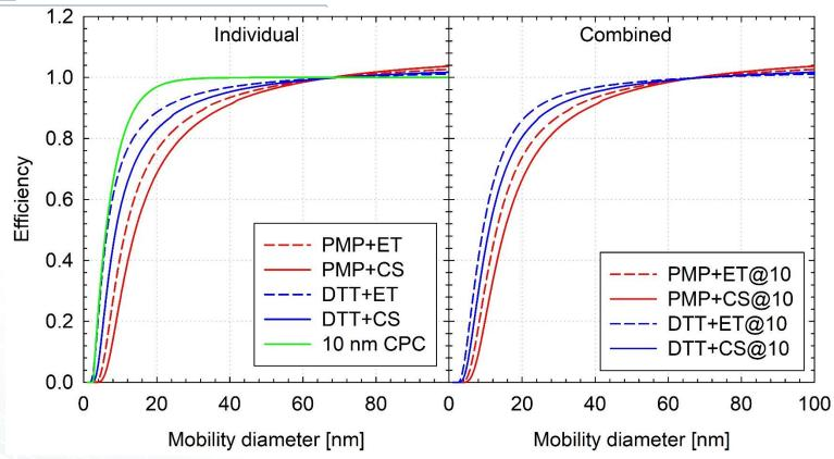
The 10 nm CPC efficiency (50% at ~7nm) is even higher than the penetration of optimized Horizon 2020 sampling systems.
