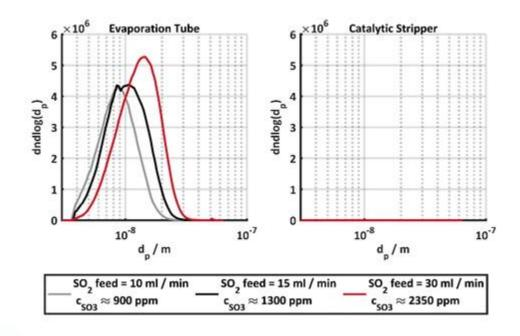
AVL's CS was found to completely suppress  $H_2SO_4$  nucleation even at excessive exhaust concentrations of  $SO_3$  (900 to 2350 ppm).
