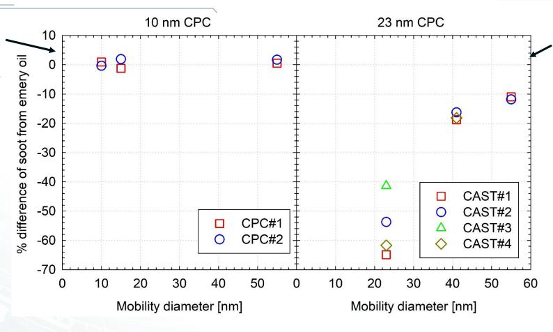
Calibration of a single CPC against an electrometer with emery oil and soot from different CAST settings
