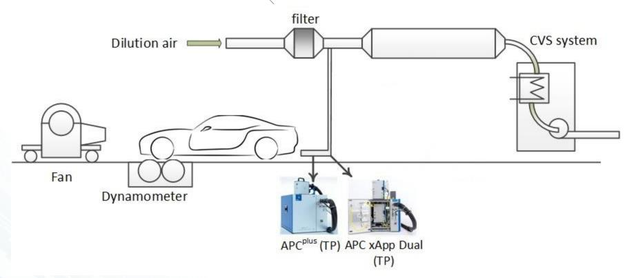
Parallel measurements with a dual line APC xApp (CS, 10 nm and 23 nm AVL CPCs) and an APC plus (ET, 23 nm AVL CPC) at the tailpipe.
