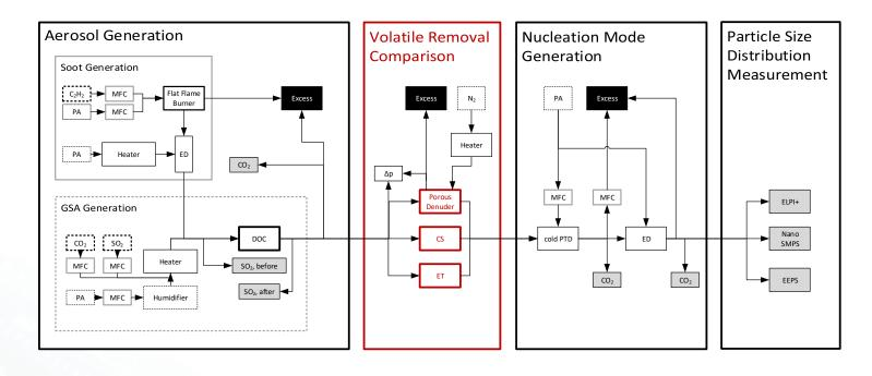
A synthetic exhaust test bench was established within DTT, able of producing controlled amounts of soot and  $H_2SO_4$  concentrations.
