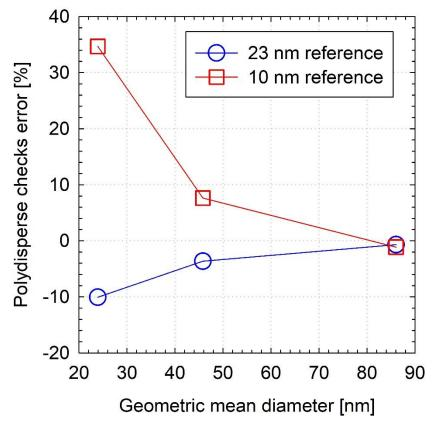
Polydisperse checks using the same 23 nm reference CPC is relatively insensitive of the losses in the system, given the high particle sampling system penetrations over the 23 nm CPC measurement range.
