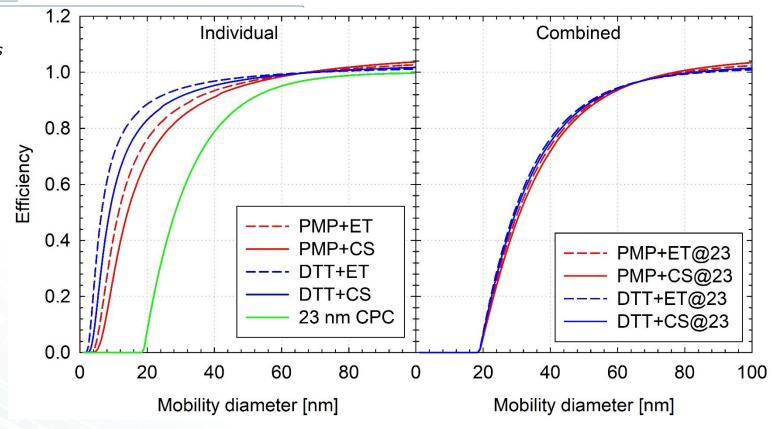
The overall (combined) efficiency of a 23 nm PN system is dominated by the low detection efficiency of the 23 nm CPC (especially for soot particles).
