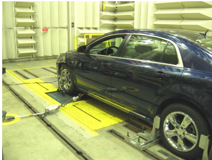
Figure 4: Test vehicle installed in on the tire noise chassis dynamometer setup for drive axis measurements
