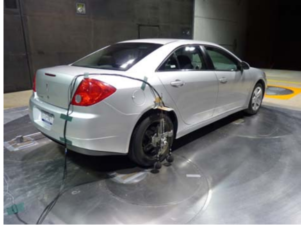
Figure 1: Pontiac G6 installed in GMAL
