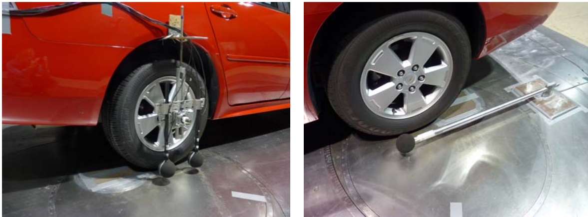
Figure 2: Vertical dual probe fixture installed on the Chevrolet Impala (left) and ideal fixture installed on the opposite side of the vehicle (right)
