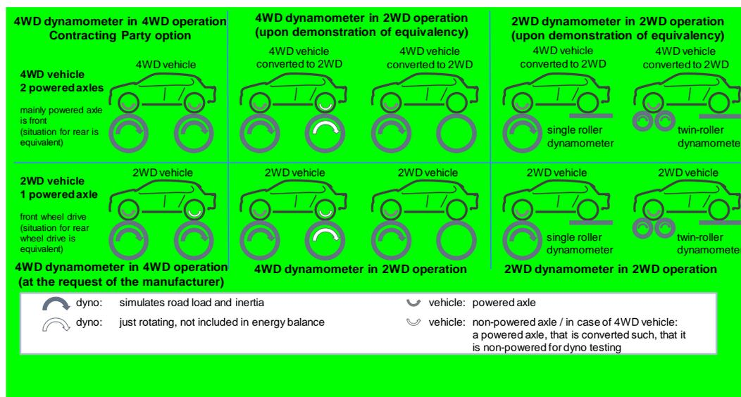
2.4.2.5. Demonstration of equivalency between a dynamometer in 2WD operation and a dynamometer in 4WD operation
