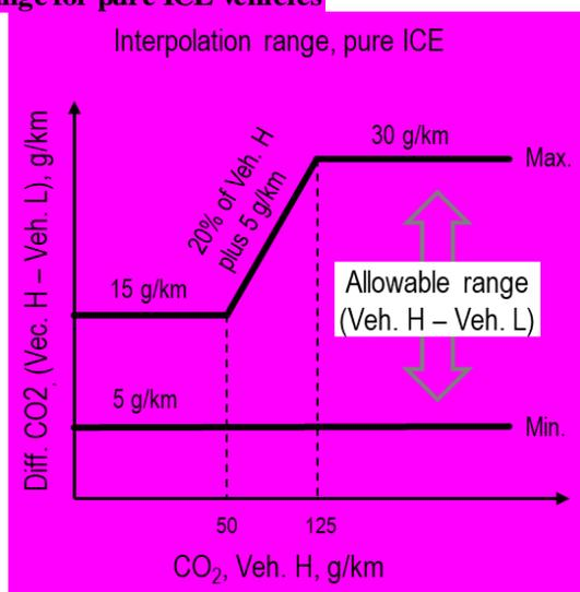
This restriction does not apply for the application of a road load matrix family or when the calculation of the road load of vehicles L and H is based on the default road load.
