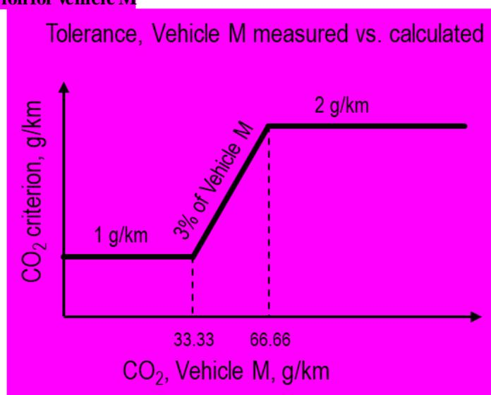
If the linearity criterion is fulfilled, the CO<sub>2</sub> values of individual vehicles shall be interpolated between vehicles L and H.
