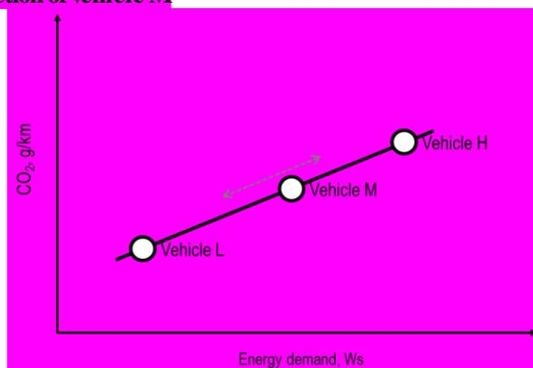
The linearity of CO<sub>2</sub> mass emission for vehicle M shall be verified against the linearly interpolated CO<sub>2</sub> mass emission between vehicles L and H over the applicable cycle by using the corrected measured values referring to the step used in Table A7/1 of Annex 7.
