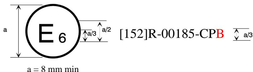
The above approval mark affixed to a vehicle shows that the vehicle type concerned has been approved in Belgium (E 6) with regard to the Advanced Emergency Braking Systems (AEBS) pursuant to Regulation No. [152] (marked with C for Car to Car, P for Car to Pedestrian, **B for Car to Bicycle**). The first two digits of the approval number indicate that the approval was granted in accordance with the requirements of Regulation No. [152] in its original form.
