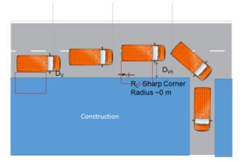
M2/N2 vehicles increases lateral distance to 1.5 to 1.9 m max at Sharp corners and in very Low speed conditions to Enable driving in very narrow single lane road
