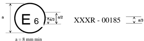
The above approval mark affixed to a vehicle shows that the vehicle type concerned has been approved in Belgium (E6) with regard to the Moving Off Information System (MOIS) pursuant to UN Regulation No. [XXX]. The first two digits of the approval number indicate that the approval was granted in accordance with the requirements of UN Regulation No. [XXX] in its original form.
