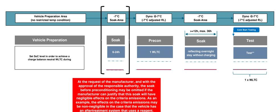
Agreed Low Temp Test Procedure for CD-test of OVC-HEV)
