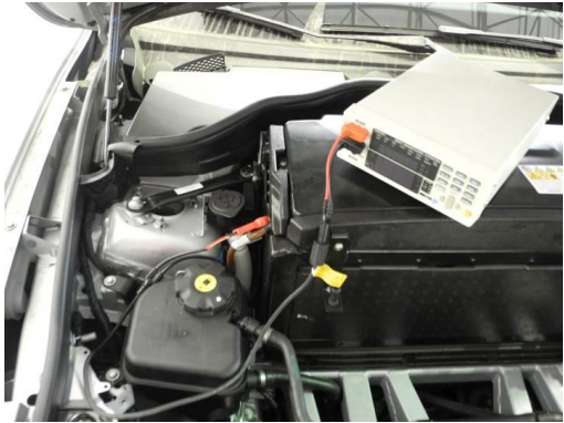
电位均衡测试 Potential equalization test
