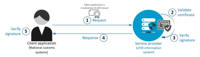
The client application (national customs systems) sends a message to the service provider (eTIR international system - Step #1). The message includes the client application's credentials, signed with the private key that is paired with the public key in the client application's X.509 certificate. The service provider validates the certificate by performing a number of checks (Step #2), including:
