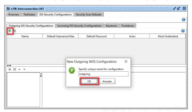
6. This configuration type is used for encryption, signing and adding SAML, timestamp and username headers. In this situation, only the signing part is used. Add a signature entry.
