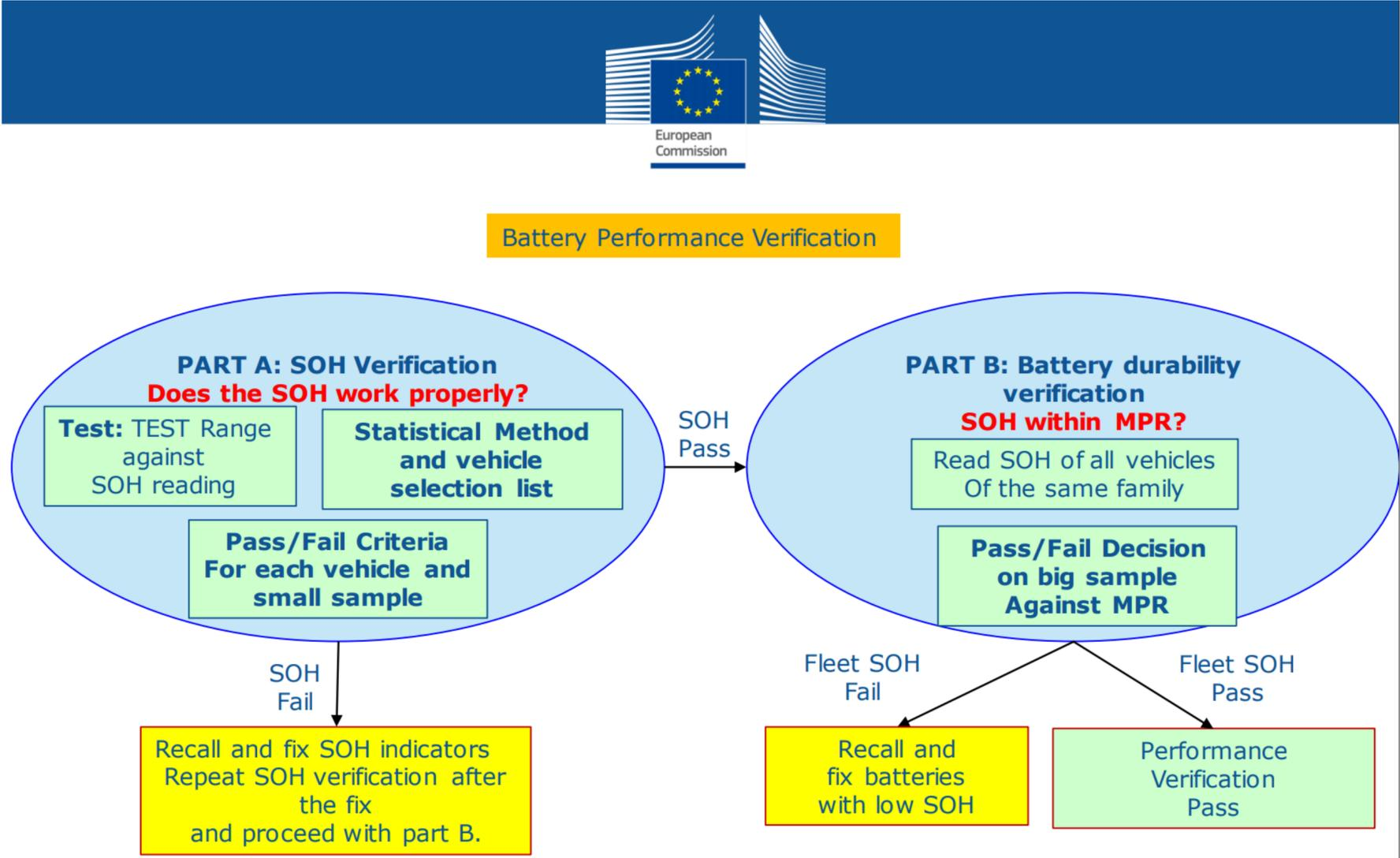
**Part A:** AVERE supports OEM choice in how SOH is measured, using the best possible SOH metric and protocol (capacity retention)
