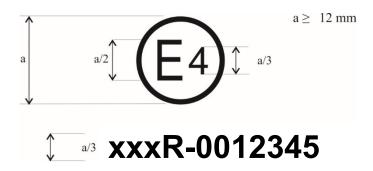
The above approval mark, affixed to a tyre shows that a tyre concerned has been approved in the Netherlands (E 4) pursuant to Regulation No. xxx, under approval number 0012345. The first two digits of the approval number (00) indicate that the approval was granted according to the requirements 00 series of amendments to this Regulation.
