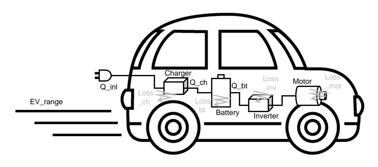
EV\_range = f(Q\_bt, Loss\_bt, Loss\_inv, Loss\_mot,)
