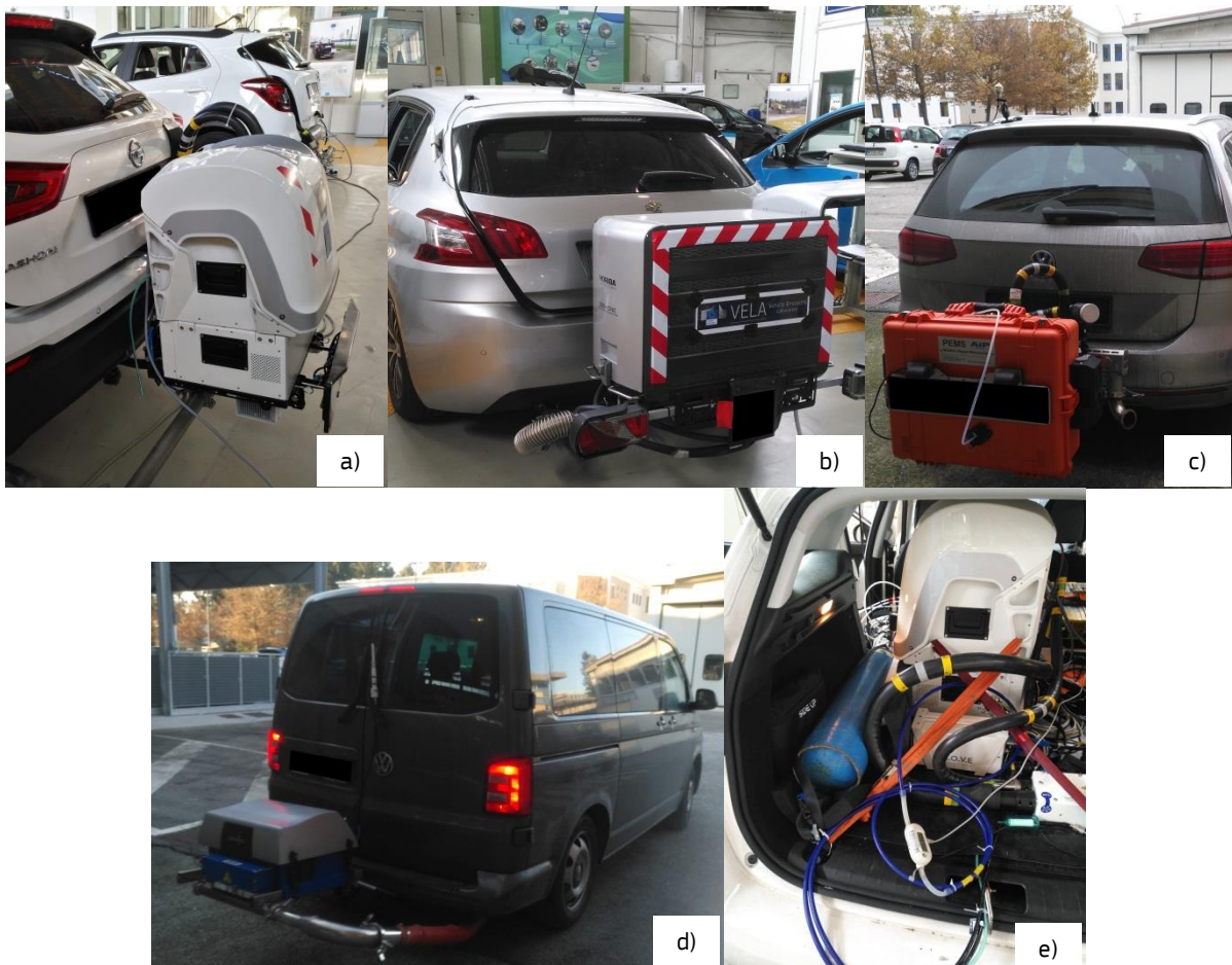
Figure 1. Overview of PEMS installations on the trailer hook for the three PEMS instruments assessed: a) AVL-MOVE, b) HORIBA OBS-ONE, c) AIP-PEMS, d) SENSORS SEMTECH LDV and e) fixation of N 2 bottle on-board the vehicle.
