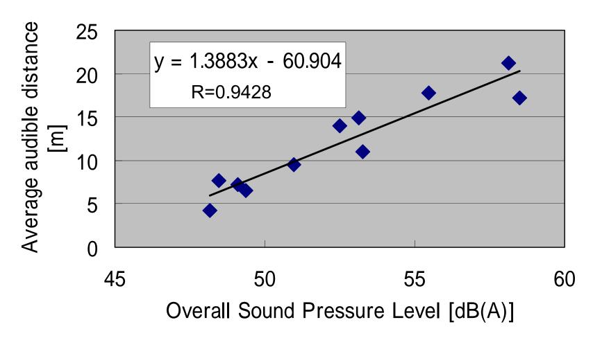
Verified audible distances of sounds with 2 bands is proportional to O.A. under condition of background noise proposed in NPRM (55dB)
