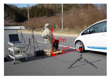
Measurement of audible distance. Participants: 12 (30 -50 years old) Approaching sounds 1/3 oct. bands: 200Hz + 2kHz, 200Hz + 5kHz,800Hz + 2kHz, 800Hz + 5kHzVolume: 46dB, 52dB, 58dB in O.A.
