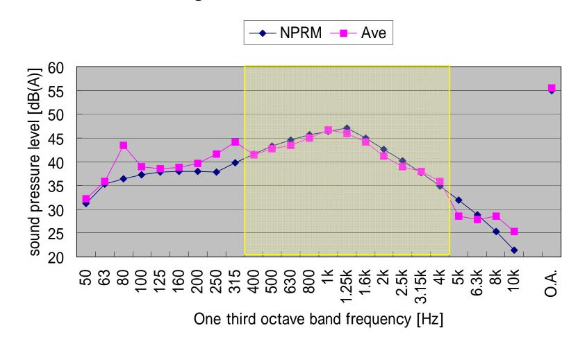
Comparison of 1/3 octave band frequency level between NPRM and averaged real-world.
