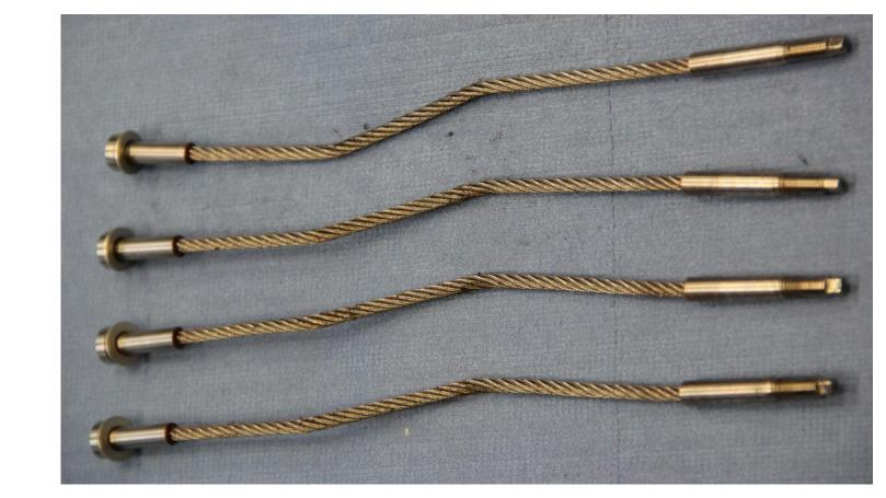
Wearing/deformation at steel cables
