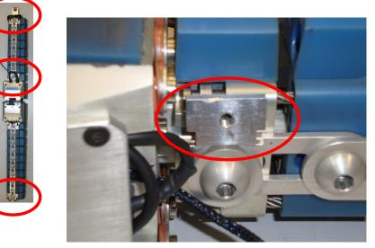
• Stress relief for trigger cable at knee element missing
