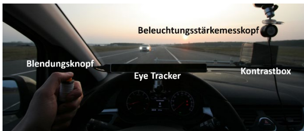
Figure 8: View from inside a measuring vehicle: blinding button, eye-tracker, contrast box and the illuminance sensor head
