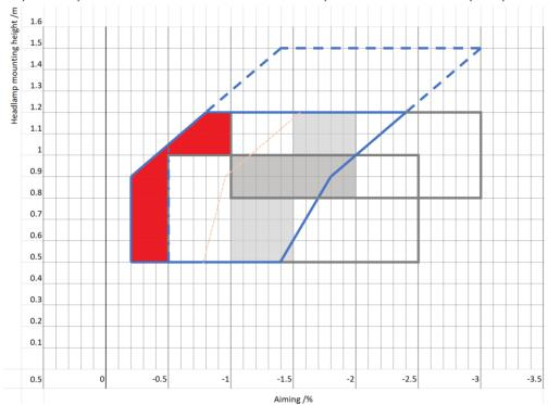
Superimposing both current and proposed R48 requirements on the same graph demonstrates the differences between the two sets of criteria.
