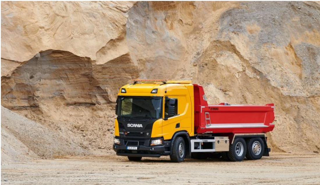
N3 construction vehicle N.B. relatively low chassis/cab height
