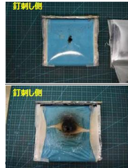
Internal cell structure after nail penetration
