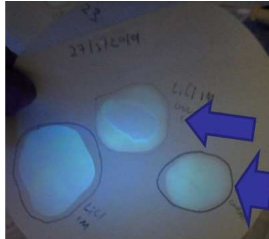
1 M LiCl (left); Coolant A (right); Coolant A + 1M LiCl, after 2 months
