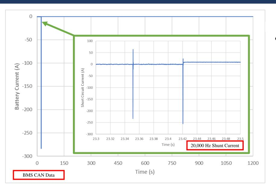
During repair of the vehicle it was determined that the fuse on the manual disconnect level was blown and a relay contactor was shorted.
