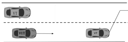
Figure 12 Schematic diagram of the front vehicle cut out test scene
