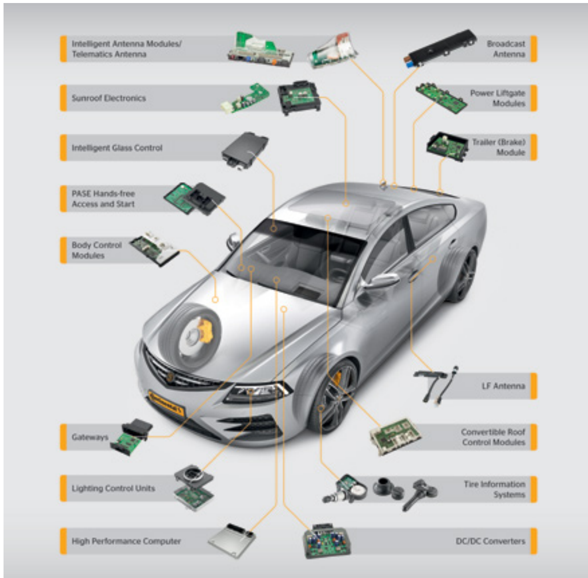
Figure 12: Various Electronic Control Units (ECUs) used in vehicles. (Source: Continental 98 )
