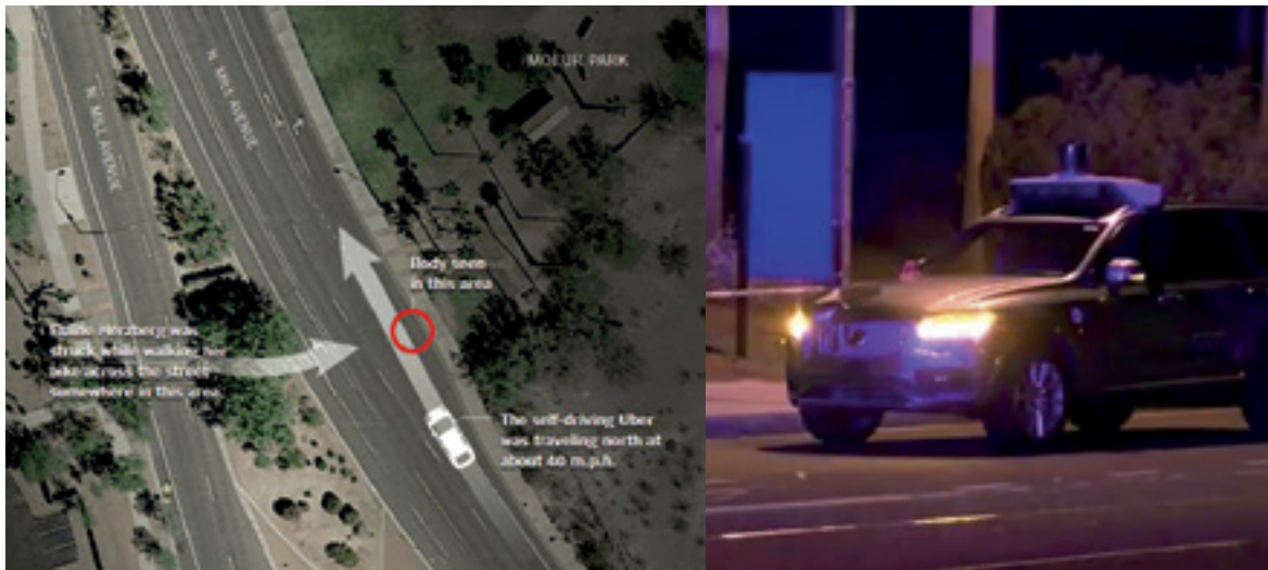
Figure 32: Accident involving a Volvo V90 owned by Uber and equipped with a self-driving system. Left: the accident location with the route of the Uber (in green) and the pedestrian (orange). Right: the Uber car after the accident with damage to the right front. (Source: ABC, Forbes)
