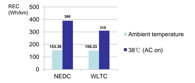
NEDC: REC increased by 154% with AC on. WLTC: REC increased by 106% with AC on.
