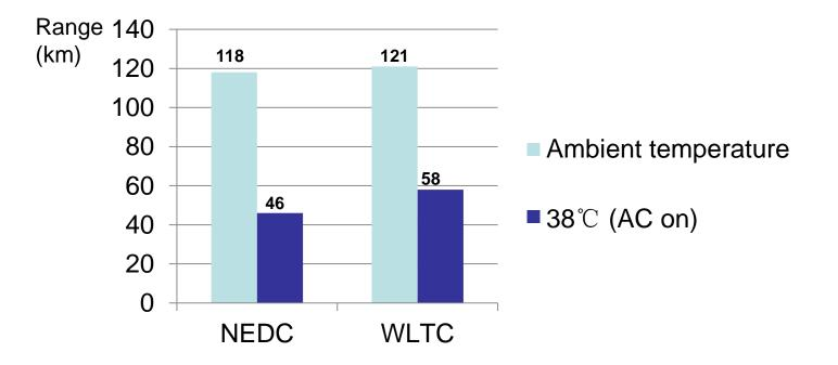
NEDC: Range was reduced to 39% with AC on. WLTC: Range was reduced to 48% with AC on.
