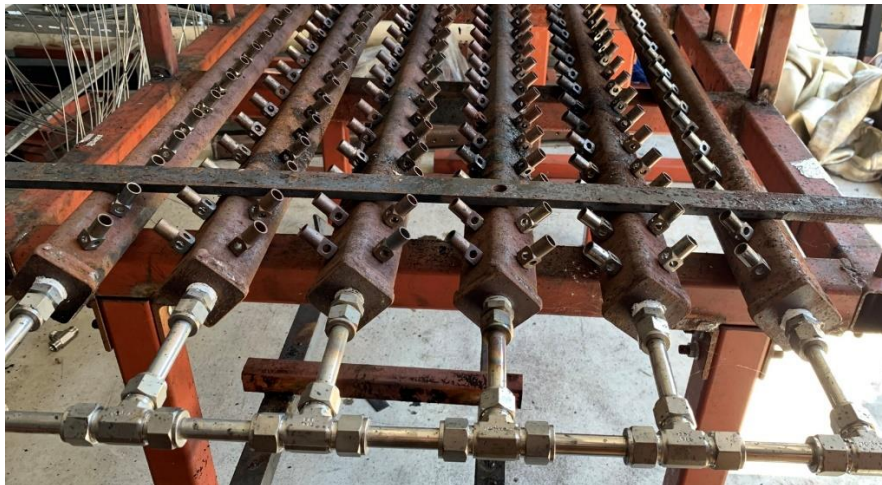
Prescribed Arrangement of Air Pre-mix Burner Nozzles
