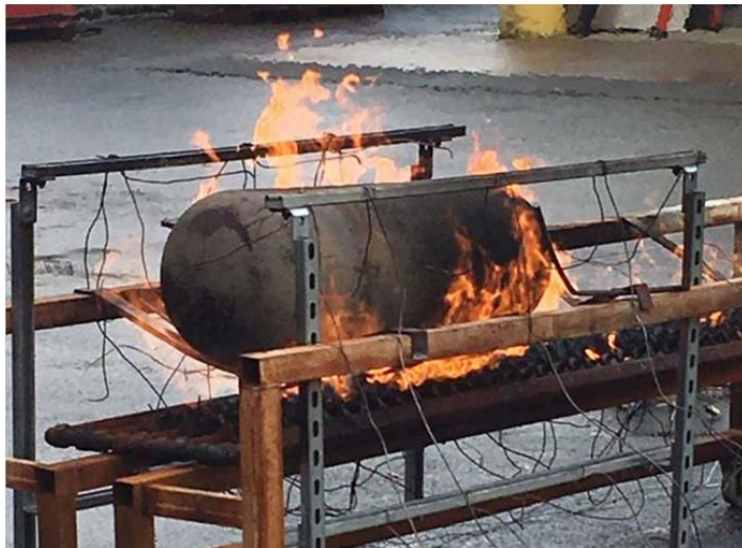
Figure 4c. Container Under-going Fire Testing
