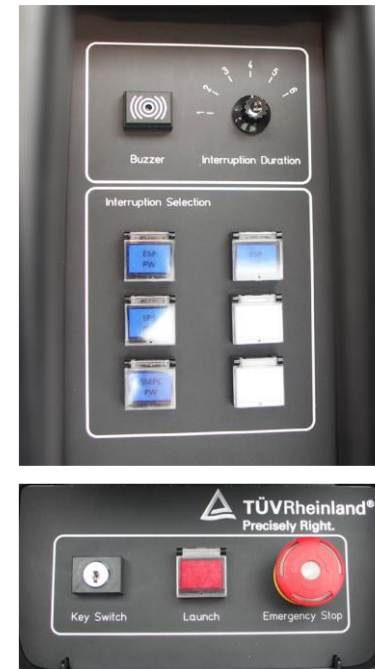
Control Unit of the ESU
