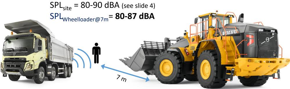
RWS: SPL<sub>Truck RWS@7m</sub> > **86 dBA => SAE J994 Type B**
