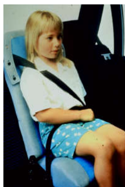
Figure 1b. Example of second-generation booster cushion from 1985, with a removable backrest
