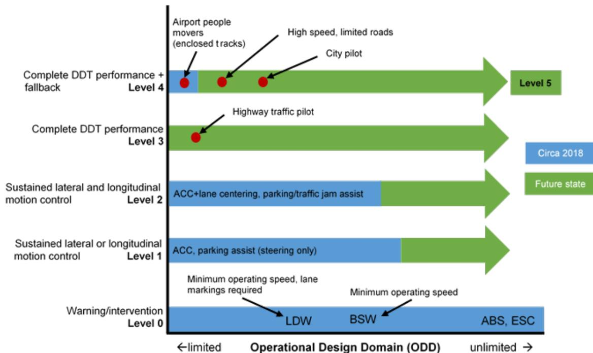
Figure 11 - ODD relative to driving automation levels
