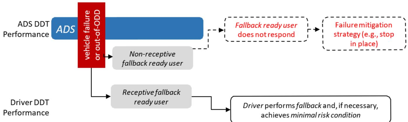
**Figure 13 - Use case sequence for a Level 3 feature showing ADS engaged, occurrence of a failure or out-of-ODD condition, and the fallback-ready user performing the fallback, or, if the fallback-ready user fails to do so, a failure mitigation strategy, such as stop-in-lane**
