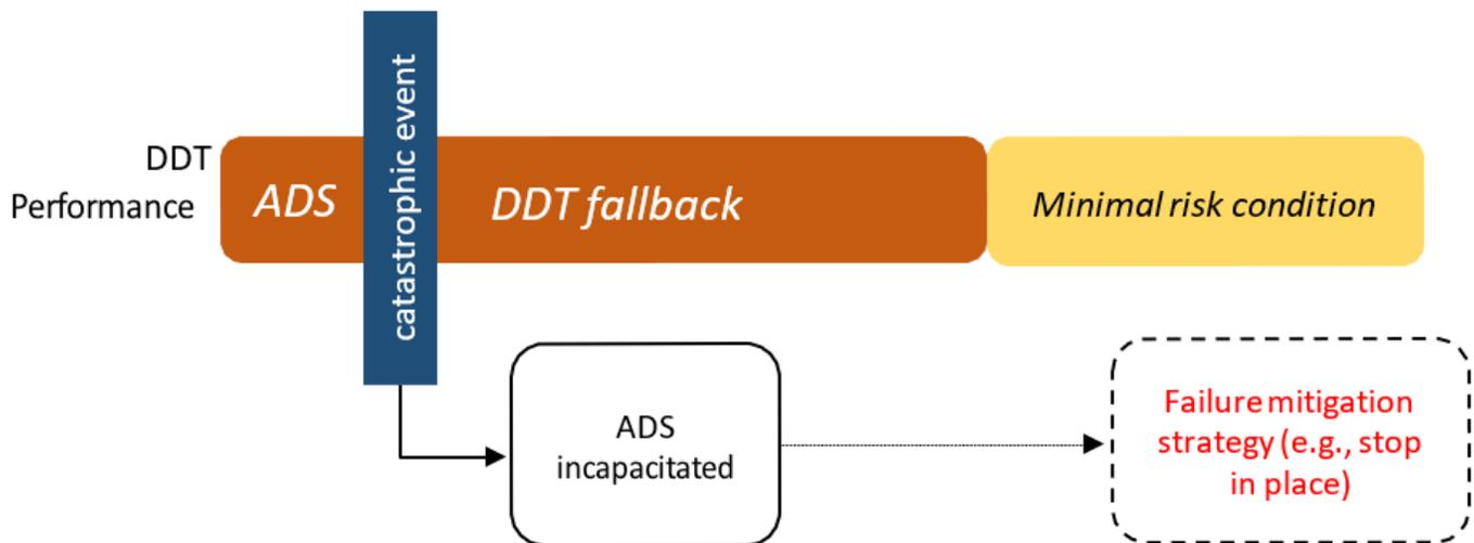
**Figure 14 - Use case sequence at Level 4 showing ADS engaged, a catastrophic event (e.g., complete power failure) and the system achieving a minimal risk condition**
