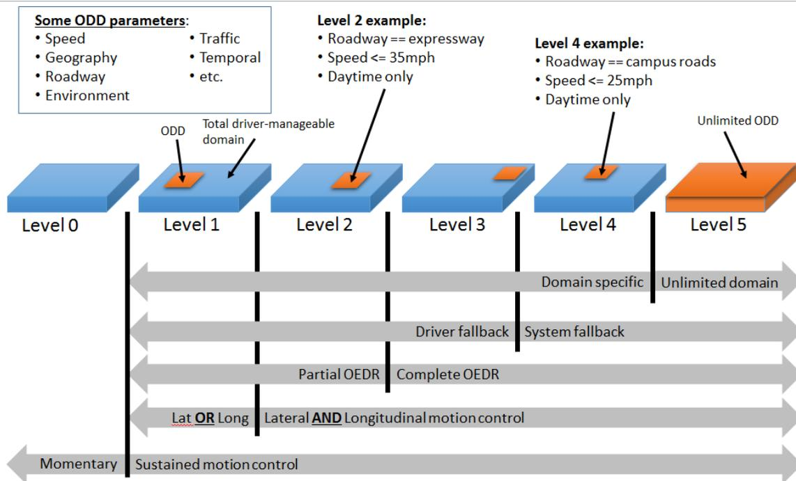
**Figure 12 - ODD relative to driving automation levels**
