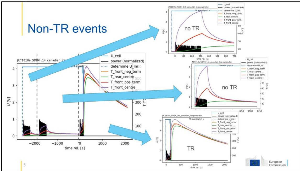
Some tests needed several starts to go into thermal runaway. These test records were split in several parts (vertical dashed lines) and the thermal events not resulting in thermal runaways were considered as independent tests. (It is acknowledged that that is not the same as starting a test with a fresh battery, e.g. inner temperature might be different.)
