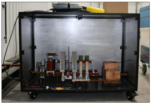
Figure 17: External Short Circuit Contactor
