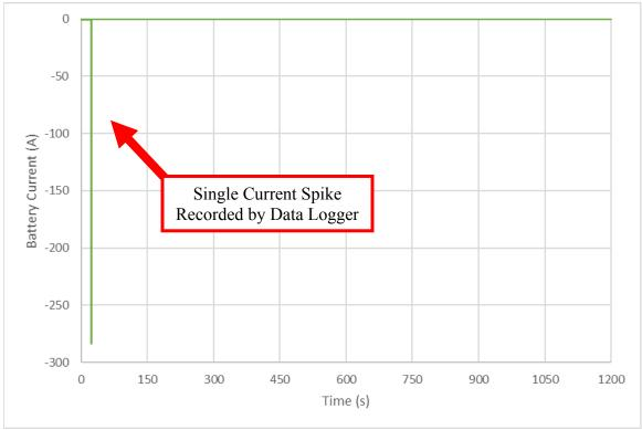
Figure 19: External Short Circuit Test Battery Current
