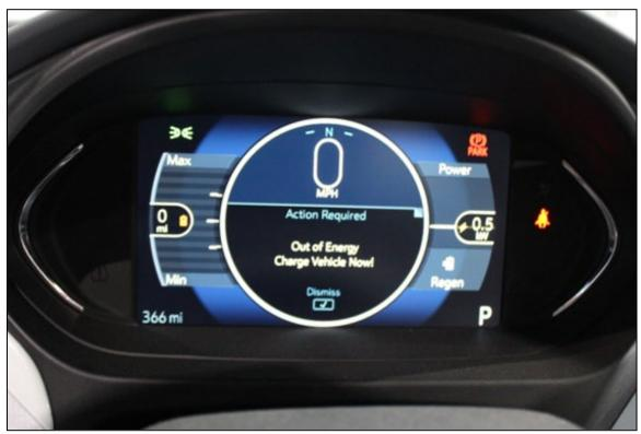
Figure 33: Over-Discharge Post-Test Instrument Cluster Message
