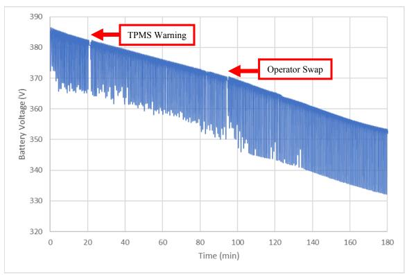
Figure 45: Over-Temperature Test Battery Voltage
