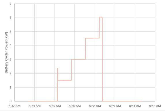
Figure 54: Over-Current Test Battery Tester Power
