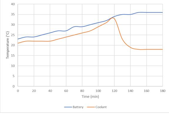
Figure 44: Over-Temperature Test Battery Temperature
