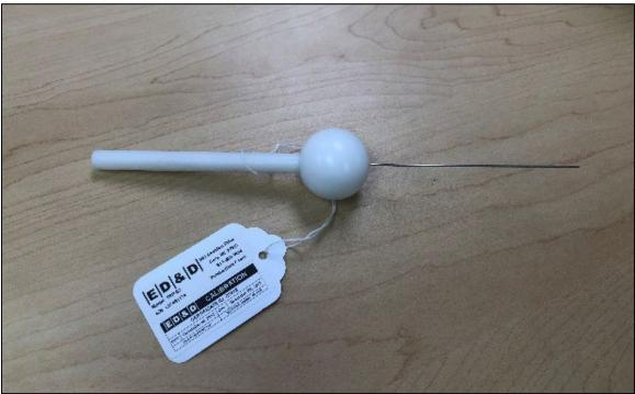
Figure 2: IPXXD Test Probe
