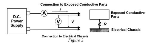
Measure the current "I" and voltage "V" between the test location and the electrical chassis. Calculate the resistance between the test location and the electrical chassis using the following formula.
