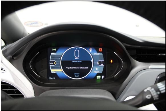
Figure 32: Over-Discharge Pre-Test Instrument Cluster Message
