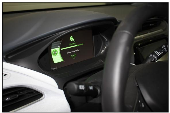
Figure 50: Over-Current Pre-Test Instrument Cluster Message
