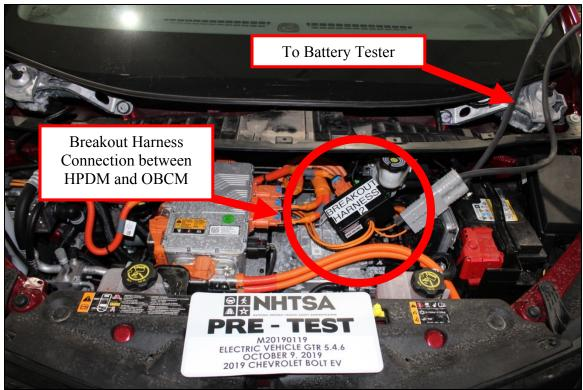
Figure 22: Over-Charge Breakout Harness
