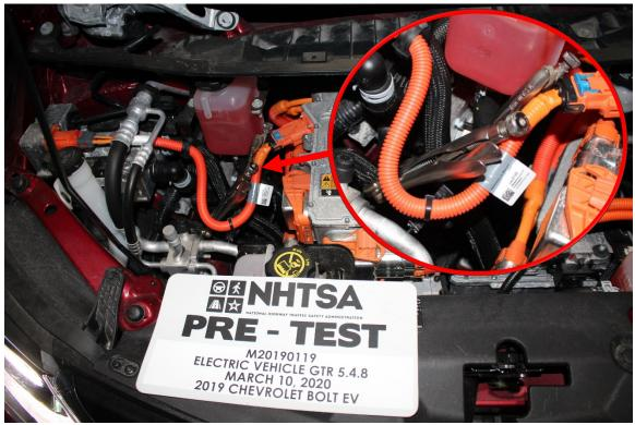
Figure 40: Over-Temperature Coolant Hose Crimps
