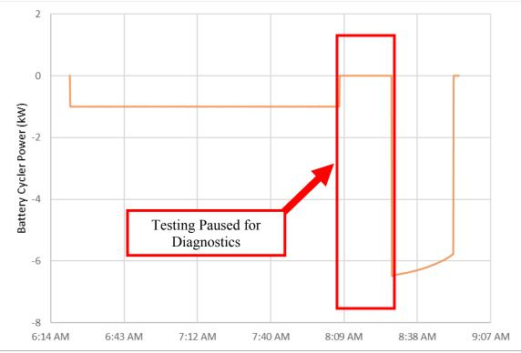
Figure 36: Over-Discharge Test Battery Tester Power
