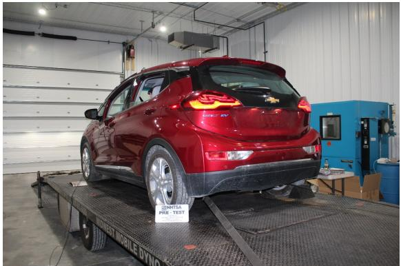
Figure 38: Vehicle Installed on Mobile Dynamometer
