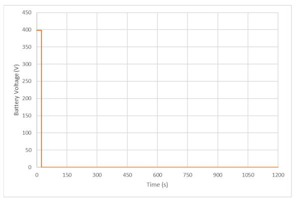
Figure 20: External Short Circuit Test Battery Voltage
