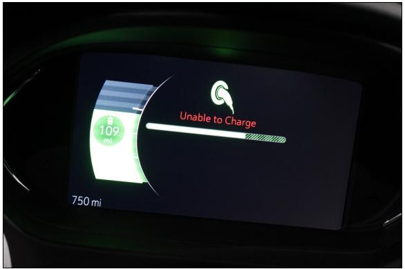
Figure 51: Over-Current Post-Test Instrument Cluster Message
