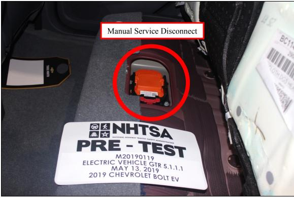
Figure 5: Vehicle Manual Service Disconnect
