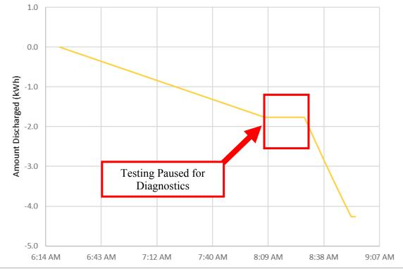
Figure 37: Over-Discharge Test Battery Tester Amount Discharged
