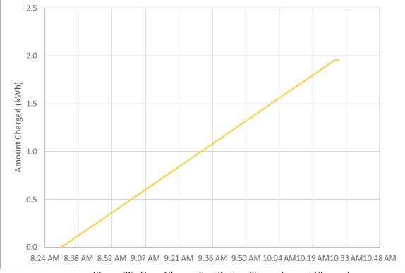
Figure 29: Over-Charge Test Battery Tester Amount Charged
