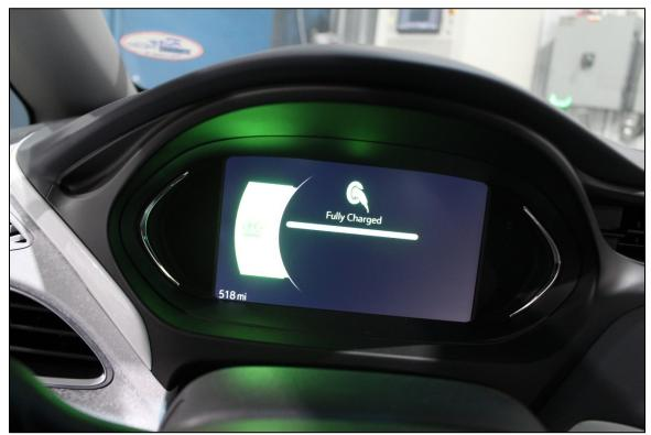
Figure 25: Over-Charge Instrument Cluster Message
