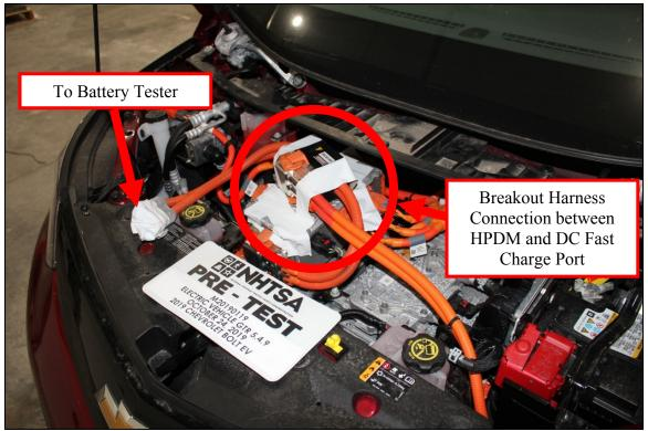
Figure 48: Over-Current Breakout Harness
