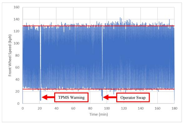
Figure 43: Over-Temperature Test Vehicle Drive Profile
