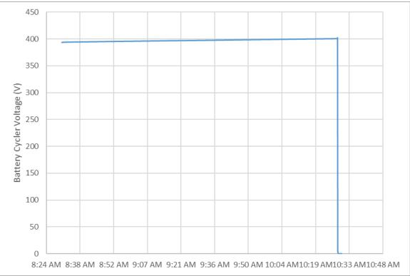
Figure 26: Over-Charge Test Battery Tester Voltage
