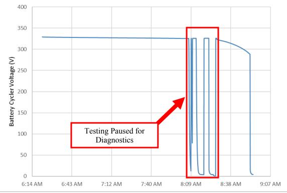
Figure 34: Over-Discharge Test Battery Tester Voltage
