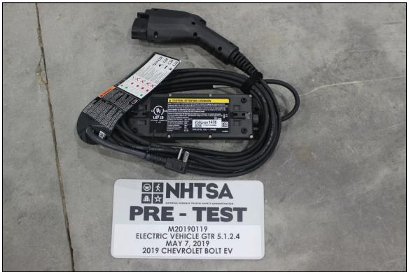
Figure 9: Vehicle Level 1 (L1) Charger
