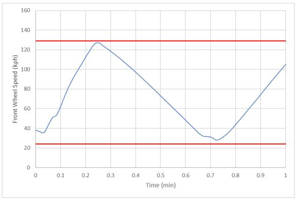
Figure 42: Over-Temperature Test Vehicle Drive Profile – Single Cycle
