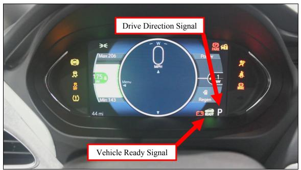
Figure 7: Vehicle Instrument Cluster
