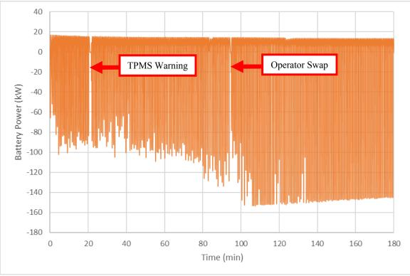
Figure 47: Over-Temperature Test Battery Power
