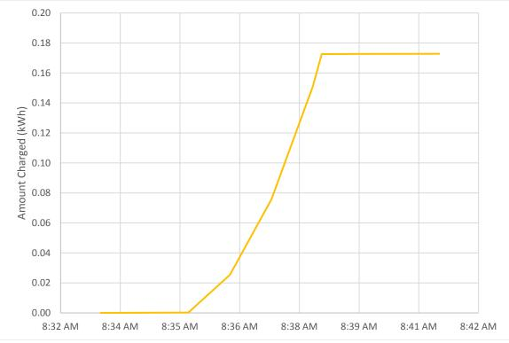
Figure 55: Over-Current Test Battery Tester Amount Charged
