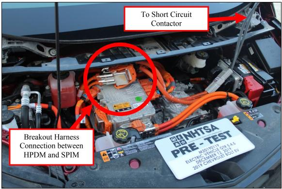
Figure 16: External Short Circuit Breakout Harness
