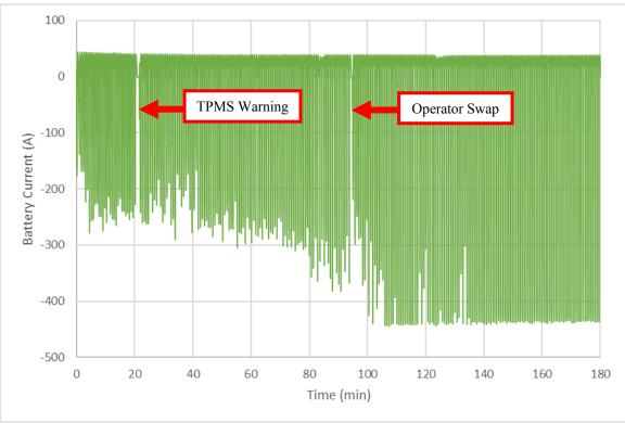
Figure 46: Over-Temperature Test Battery Current
