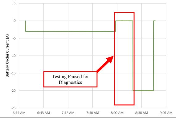
Figure 35: Over-Discharge Test Battery Tester Current
