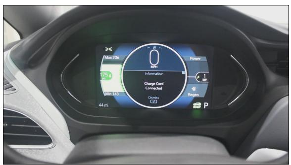
Figure 12: Signal to Driver When Selecting Active Drive Mode Possible While External Charging Is Active.
