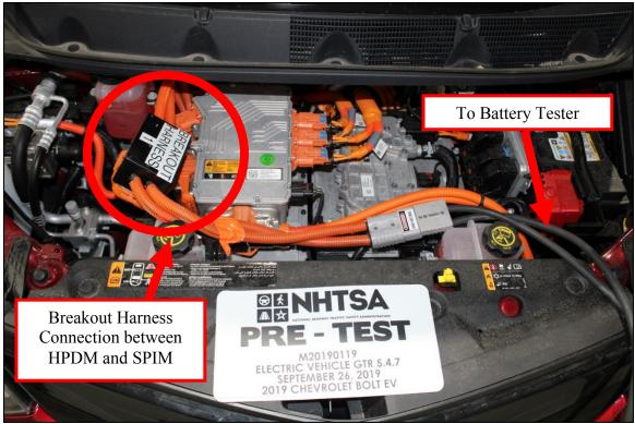
Figure 30: Over-Discharge Breakout Harness
