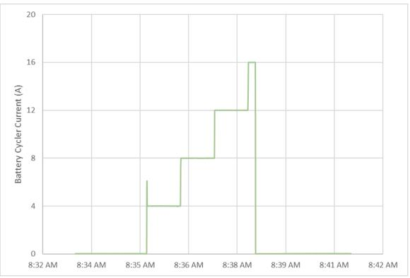
Figure 53: Over-Current Test Battery Tester Current
