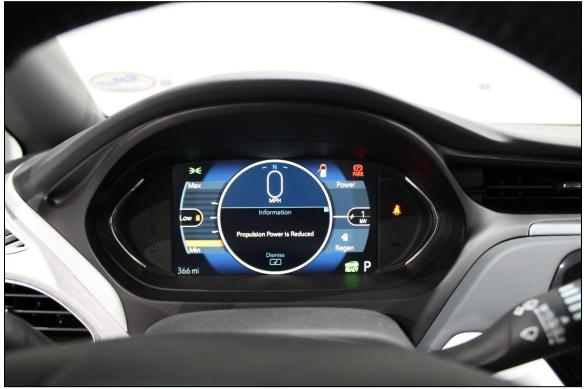
Figure 13: Low Energy Warning to the Driver
