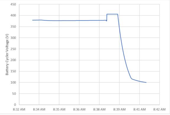
Figure 52: Over-Current Test Battery Tester Voltage
