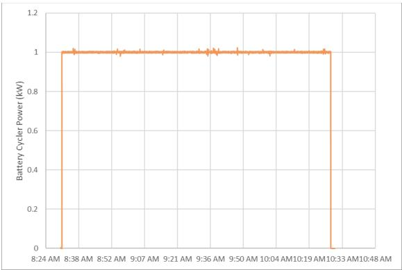
Figure 28: Over-Charge Test Battery Tester Power
