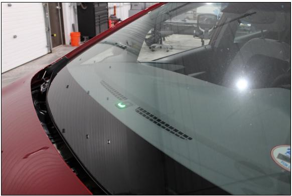
Figure 24: Over-Charge Dash Indicator Light
