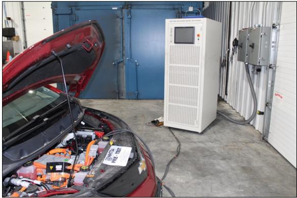
Figure 31: Over-Discharge Test Setup
