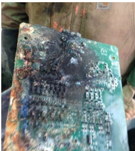
Figure 2. Fisker Karma Flooding – BMS and internal cabling damage and shorting
