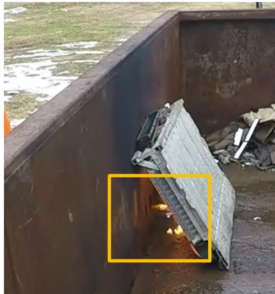
Figure 12. Location of direct flames for initiation of battery incineration
