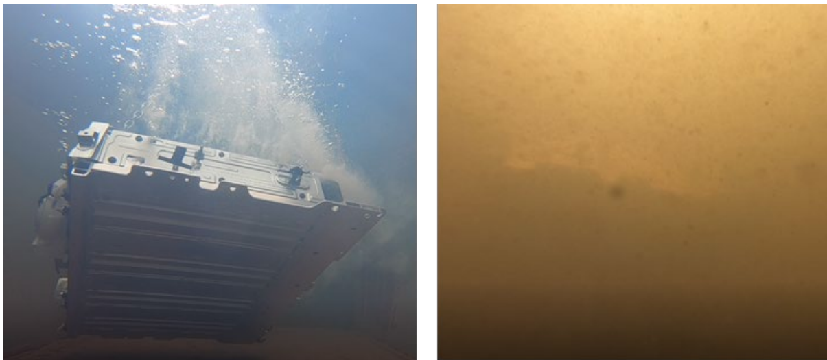
Figure 10. Underwater camera view during immersion (left - initial immersion, right – approximately eight minutes after immersion)
