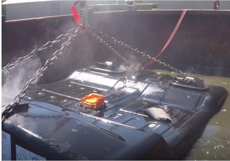
Figure 24. BEV (Test #3) battery showing smoke during observation period
