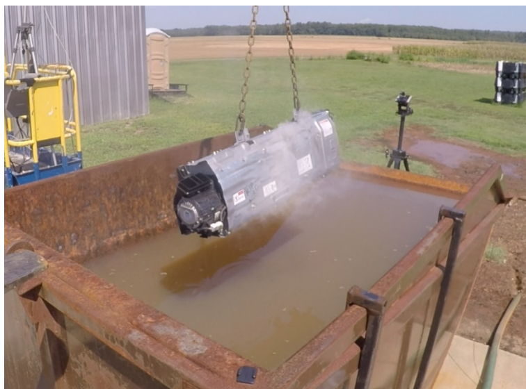
Figure 25. PHEV (Test #7) battery showing smoke during observation period
