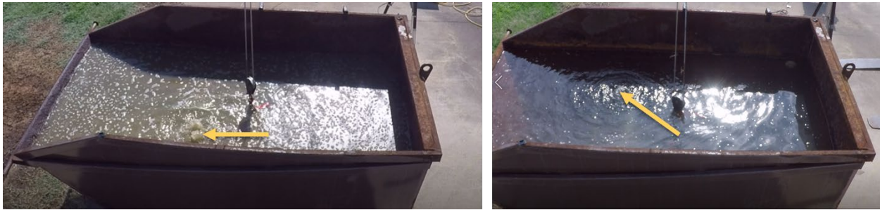
Figure 23. Battery reactions after 5 minutes of immersion in seawater (left) and brackish water (right)
