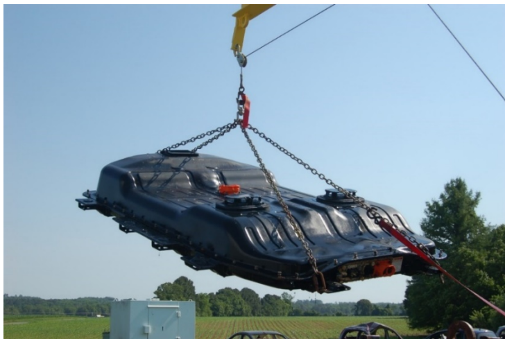
Figure 15. Angled battery prior to immersion (to avoid floating)
