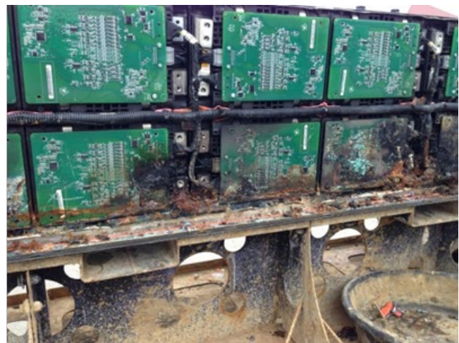
Figure 2. Fisker Karma Flooding – BMS and internal cabling damage and shorting
