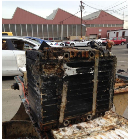
Figure 3. Fisker Karma – evidence of actual individual cell damage
