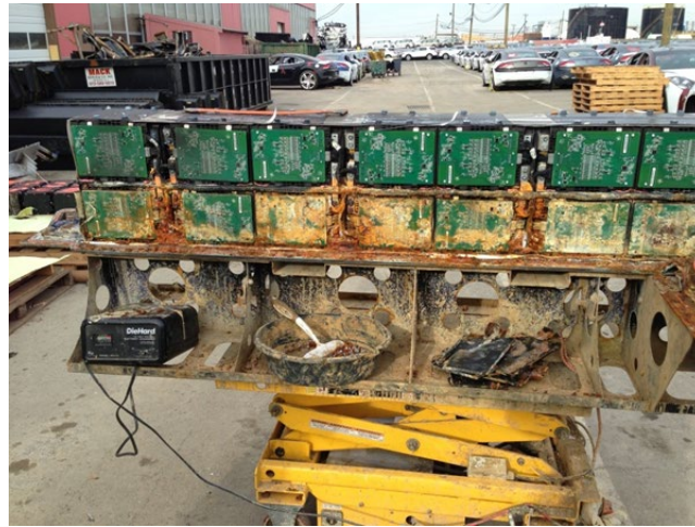
Figure 1. Fisker Karma Flooding – water intrusion of the
