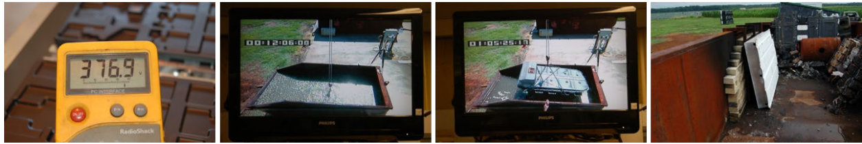
Figure 14. Overview of battery immersion testing process - Battery preparation, immersion, observation above immersion tank and extended observation
