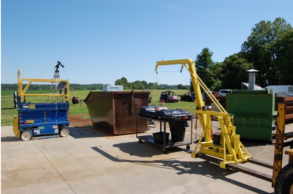
Figure 4. Test setup overview – observation station, lifting mechanism, and immersion tank
