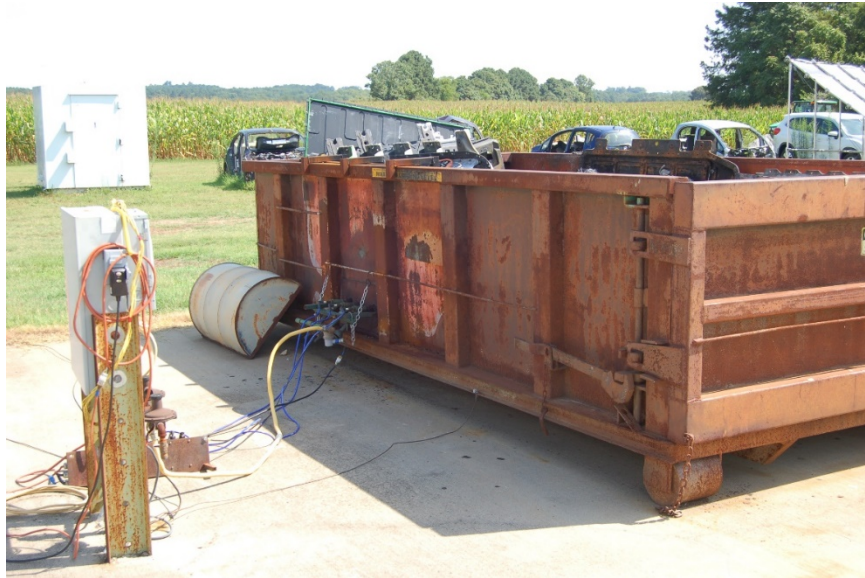
Figure 11. Secondary containment for long-term observation and final battery destruction
