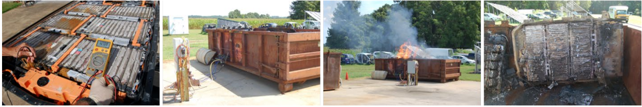
Figure 16. Overview of final battery destruction process
