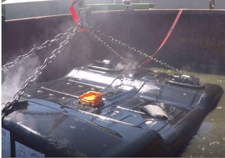
Figure 9. Waterline immersion tank camera view
