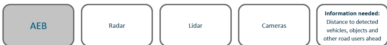
Figure 4 AEB most used sensor types and input.
