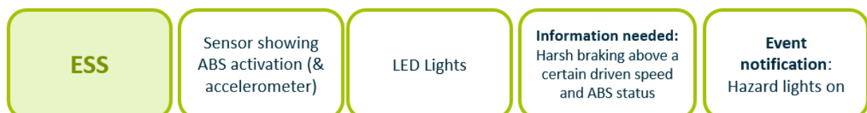
Figure 6 ESS's sensors, input and event notification (to the following vehicle).
