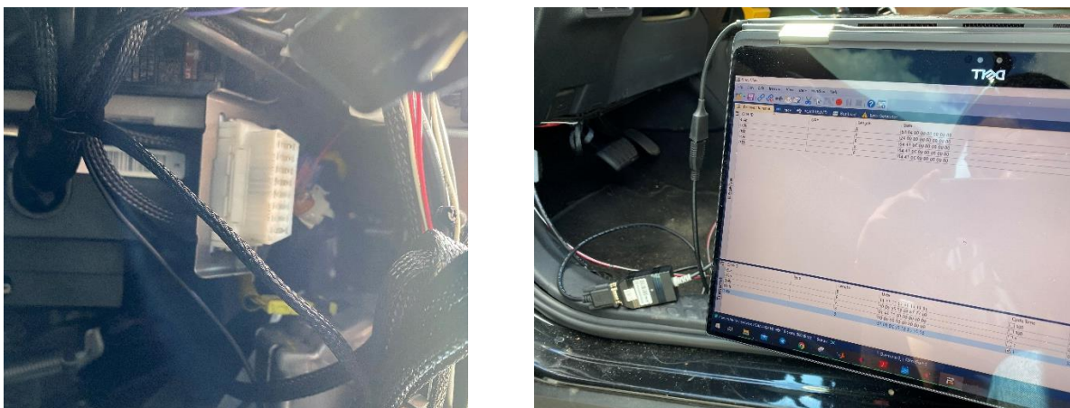
Figure 19 Left: eOBD port, Right: Data logging through PEAK CAN.
