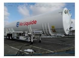
Low temperature, vacuum insulated tanks
