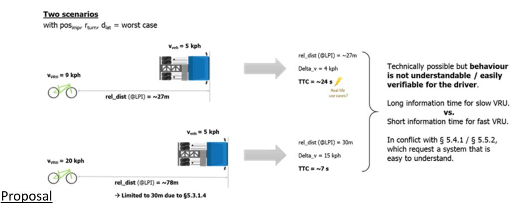
Similar to limitation of the FoV (30m to the rear and 7m to the front) we propose to limit the TTC. The value must be decided within the VRU Proxy group. Example: "Information signal shall be provided, at least, when a potential collision with cyclist is less than [X] TTC"
