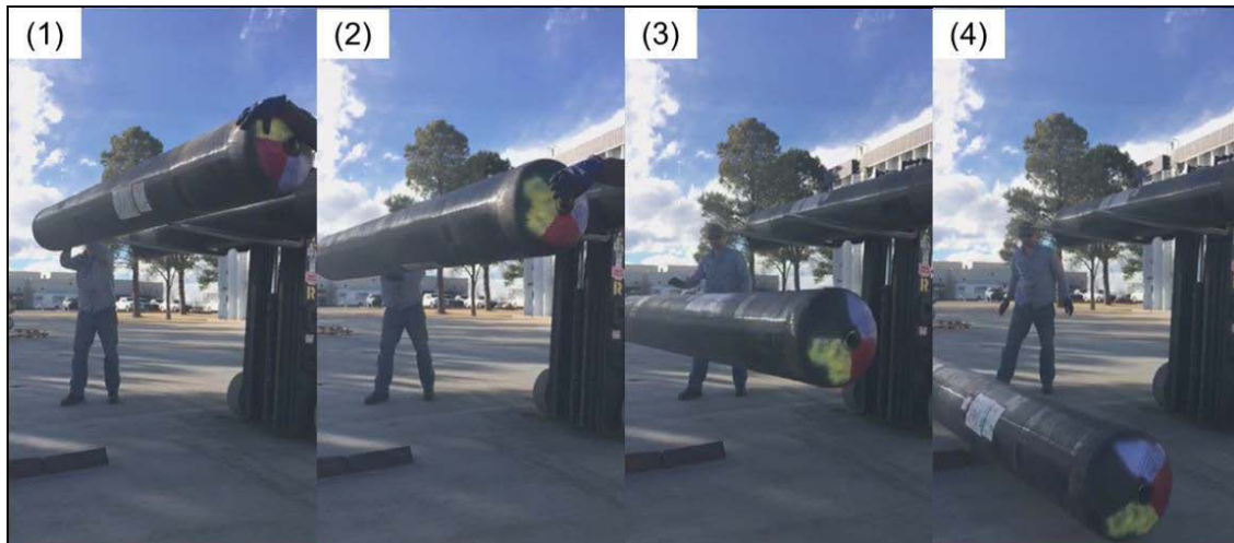
Figure 4. (1) Tank at testing height; (2) drop initiation of the tank; (3) tank dropping; (4) impact of the tank onto the steel angle iron
