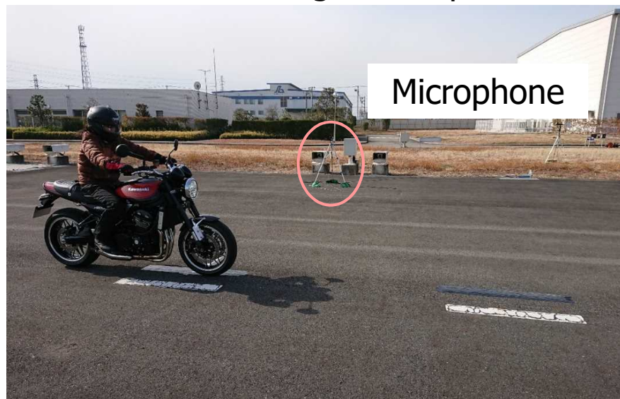
Measurement of training data at test site
