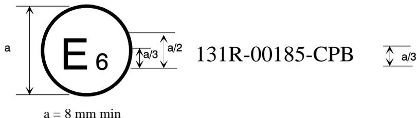
The above approval mark affixed to a vehicle shows that the vehicle type concerned has been approved in Belgium (E 6) with regard to the Advanced Emergency Braking Systems (AEBS) pursuant to UN Regulation No. 131 (marked with C for Vehicle to ~~Car~~ **Vehicle**, P for Vehicle to Pedestrian, B for Vehicle to Bicycle). The first two digits of the approval number indicate that the approval was granted in accordance with the requirements of UN Regulation No. 131 in its original form.
