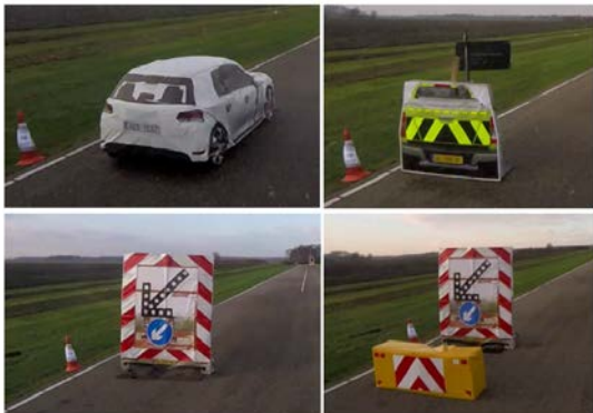
Figure 10 - The slab foam targets in four different layouts: representing a car (upper left), a road inspector vehicle (upper right), a traffic arrow trailer (lower left) and a collision absorber (lower right).
