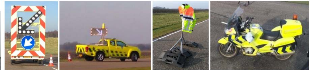
Figure 1 Traffic control measures tested: traffic arrow trailer, WIS car fend-off, WIS jacket, WIS motorcycle. [3]
