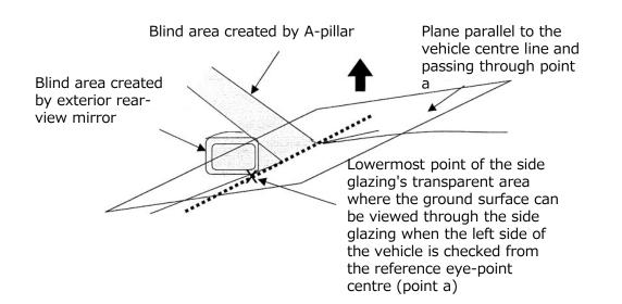
The range of the blind area created by the A-pillar or exterior rear-view mirror in paragraph 15.2.4.10. shall be an area that meets the following formula. In this case, if there are more than one blind area, each blind area shall meet the conditions of the formulae.
