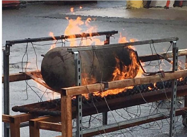
Figure 4c. Container Under-going Fire Testing
