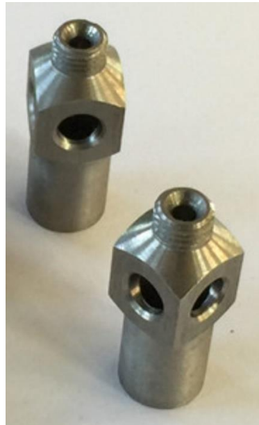
Figure 4f Burner Fuel Nozzles
