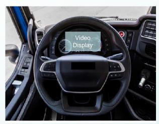
The monitor defined size shall be visible without any obstruction from the ocular reference point.
