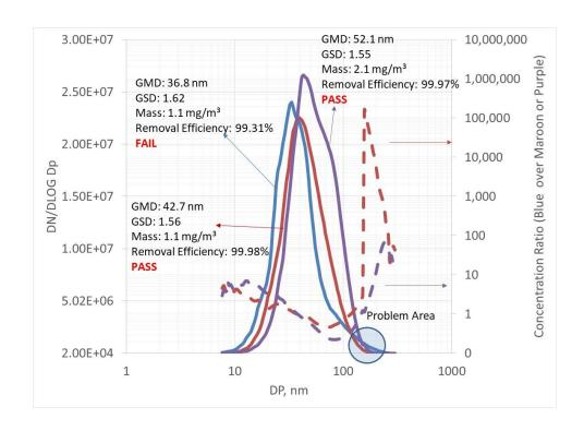
If the inlet concentration is 1e7 part./cm<sup>3</sup> at a dilution ratio of 100, all you need is >100 part./cm<sup>3</sup> to survive and fail the removal efficiency. The cause for the failure is typically surviving particles with a size around 10 to 15 nm in diameter.
