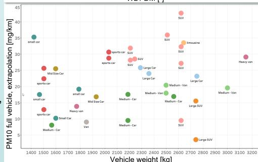
a.auto <sup>1</sup> full-vehicle emission values are calculated from single brake results as 3 x front axle or 6 x rear axle.
