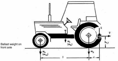
5.2.1 All tractors with a loaded mass exceeding 2,5 tonnes must be fitted with a trailer coupling having a ground clearance satisfying one of the following relations:
